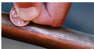
If when scratched the pipe is orange and shiny like a penny, your pipe is made of copper. A magnet will not stick to it.
