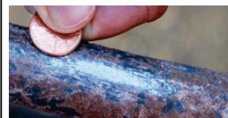
If the pipe is silvery gray and, 1) is easily scratched, 2) the metal seems soft, and 3) a magnet doesn't stick to it, you likely have a lead pipe.
