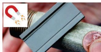
If the pipe is silvery gray and hard to scratch, place your magnet on it. If the magnet sticks, your pipe is galvanized steel or galvanized iron.
